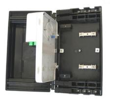
Horizontal fiber splice closure FOSC4809 is designed with both butt-joint, branching and splitting and wiring function. It has max 48 fiber capacity and suitable for main bunchy optical cable and different diameter drop cables.
