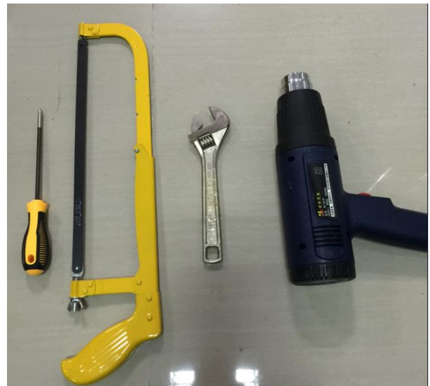
2. Prepare installation tools well (screwdriver, hacksaw, wrench, hot-air blower)
