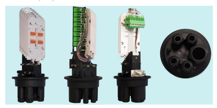
The dome fiber optic splice closure GPJM5-JF is mechanical sealing FOSC dome series with IP safety rate IP68. The dome closure is suitable for different branch connection methods including uncut cables branching, it can be installed 1x2:32 splitter or 2x2:16 PLC splitter with adapter plates The GPJM5-JF with features such as excellent sealing performance, easy for installation, wide applications.
