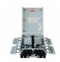
Fiber optic access terminal box FAT-R16 is designed for FTTx network application with waterproof protection level at IP-65 to hold up to 16 subscribers and 120 splicing point. ABS+PC material case provides solid protection for feeder cable splicing, distribution, splitting, storage, and connection.
